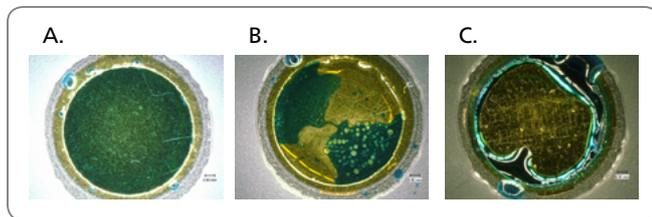
**Figure 3.** Development of a homogeneous heat-treated silicone coating on gold quartz crystals. The surfaces are covered with testing ink. A. gold-coated quartz crystal. B. inhomogeneous silicone coating, manually coated. C. homogeneous silicone layer, spincoating.
