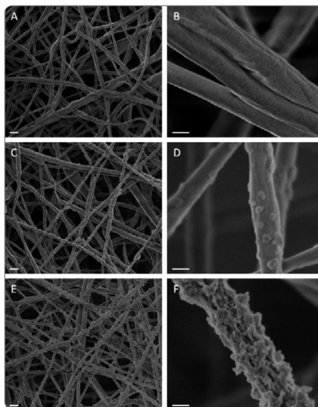
**Figure 1.** SEM visualization at different magnifications of the electrospun PCL nanofibers A,B) before LbL treatment, C,D) after the deposition of (PLL/BMP-2)<sub>3</sub> spheroid nanoarchitectures, and E,F) after the deposition of (CHI/BMP-2)<sub>3</sub> fish scale-like nanoarchitectures. Scale bars: A,C,E) 1mm and B,D,F) 100 nm [2].
