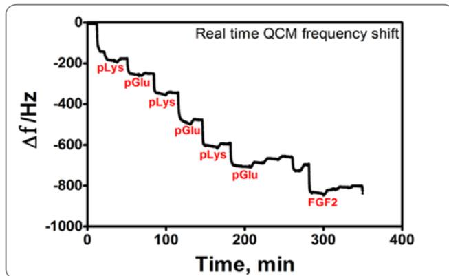
**Figure 2.** Real time QCM frequency shift ( $\Delta f$ ) upon formation of the film (pLys/pGlu)<sub>3</sub>/FGF2 on a 3-mercaptopropionic acid coated on a 10 MHz QCM resonator at 25 °C.
