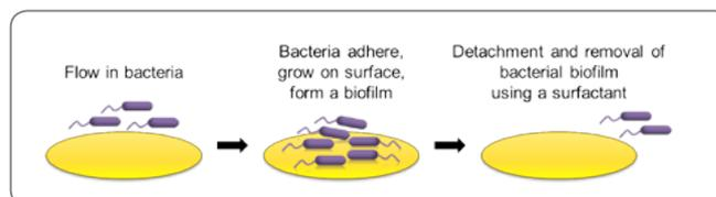
**Figure 1. Bacterial detection scheme using a quartz crystal microbalance to monitor the growth and removal of bacteria from the gold-coated sensor surface.** Using a flow cell, bacteria enter the system and attach to the gold-coated surface. Bacteria are left to grow in either stagnant conditions or under continuous flow with growth media added. After several hours of bacterial growth and biofilm formation, a surfactant is introduced to detach and remove bacteria from the surface.
