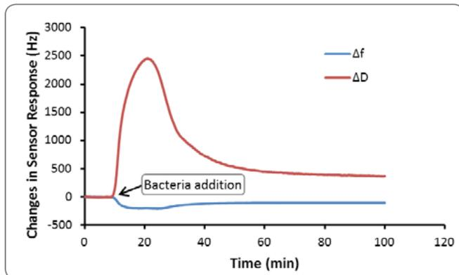
**Figure 2.** Frequency (blue) and damping (red) traces of bacterial cell deposition. *P. aeruginosa* bacterial cells are added once a stable baseline is reached for the growth media. The cells take approximately 1 hour to adhere to the gold surface and reach equilibrium.
